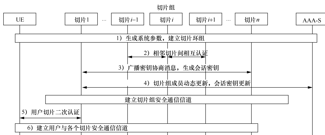
图7 5G mMTC 用户同时访问多个切片服务的协议框架 Figure 7 Framework for 5G mMTC users to simultaneously access multiple slicing services
